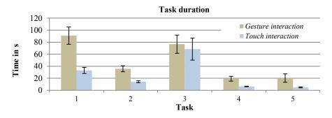
Fig. 4: Comparison of the duration of tasks with freehand gesture and touch screen interaction.
