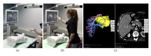
Fig. 2: Experimental setup with touch screen, plastic drape, surgical table and Leap Motion Controller (below hand, (a)). A user is performing tasks with freehand gestures (a) and touch screen interaction (b.) A screenshot of our prototype is shown in (c).
