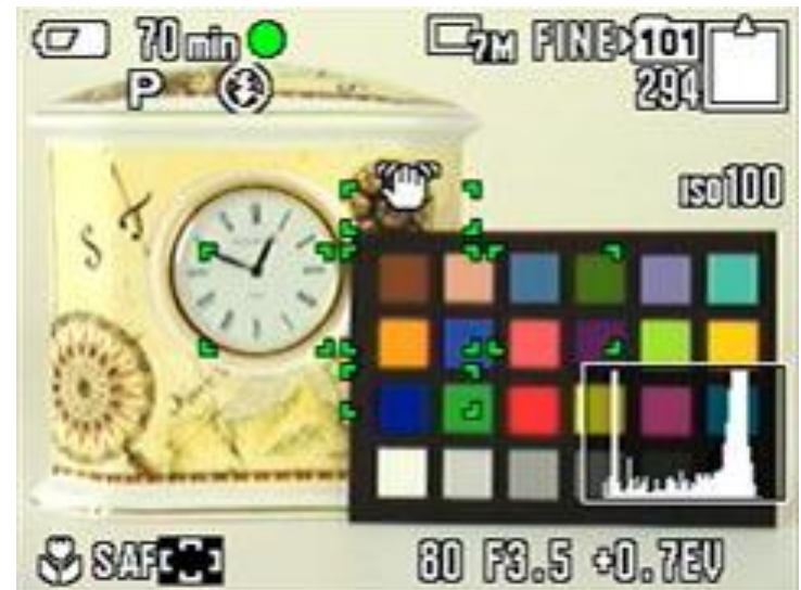
Sony DSC-V3 camera including luminance histogram (from www.dpreview.com )
